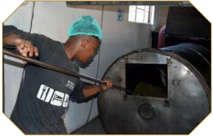
Fermenting the plant material: Quinzano Willeman is overlooking the process of heating up honeybush plant material in a stainless-steel drum for 70 hours at 70°C on the farm Nooitgedacht. Photo by Heilie Combrink, courtesy of Netwerk24 .
